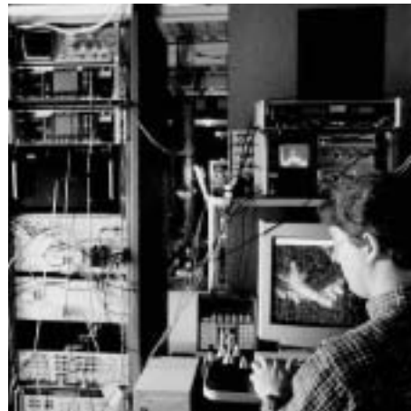
▲ Guy Demartinis, one of STL's radar engineers, evaluates the high-resolution terahertz imagery of a scaled aircraft.
